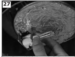
Install 1  $\times$  100 halogen bulb E-11. Do not touch bulb surface as oily residue from skin can cause the bulb to explode.
